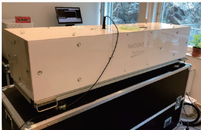
The DOAS enclosure and optical gas cell enclosures
