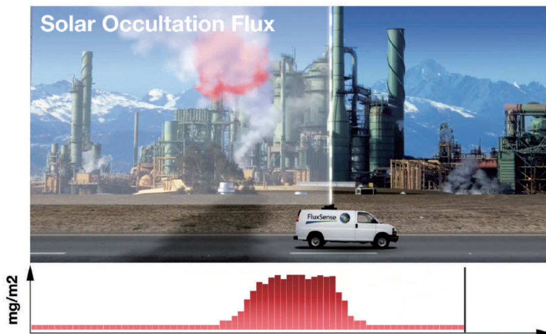
In the Solar Occultation Flux method (SOF) gases are measured by observing solar light in the infrared portion of the solar spectrum
